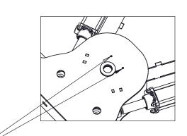
ANGLE HOLDING PIVOT POINT TYPE OF LUBRICATION: GREASE QUANTITY: 6 STROKES
