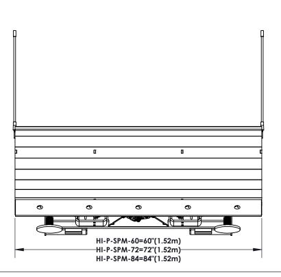
1/4" Plates construction with 3/8" quick attach mounting plates
