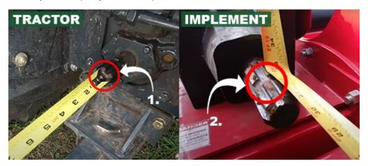
You must measure from the same two points with the implement placed in three different positions. If you plan to use a Quick-Hitch or other easy change system, this must be affixed to your tractor to ensure an exact length for your PTO shaft.
