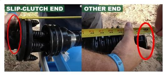
Separate the two individual pieces of the PTO shaft – you will need to remove the same distance from each half of the shaft. **Do not halve the necessary distance into two equal parts to reach the final length.**
