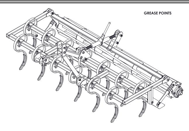
**HCF209-28 4-bolt flange bearing** TYPE OF LUBRICAION:- GREASE QUANTITY:- 4 STROKES
