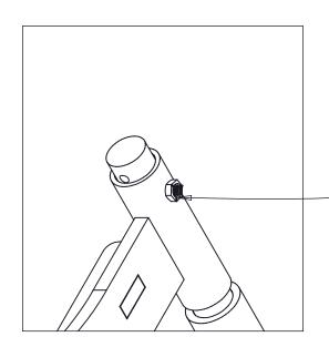
WHEEL KIT SLEEVE TYPE OF LUBRICATION: GREASE QUANTITY: 2
